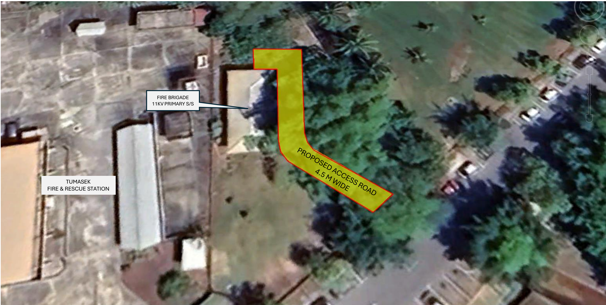
CONSTRUCTION OF ACCESS ROAD AT FIRE BRIGADE 11KV PRIMARY SUBSTATION
